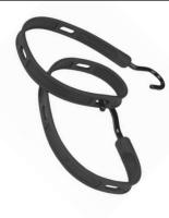
Heavy duty strap that will not break or degrade under the harshest environments including UV, ozone, gasoline, diesel fuel, oils, and even extreme temperature variations. Made from a proprietary blend of polyurethane that is guaranteed for life. The recommended stretch is 2 times the material length. Rounded hook ends are glass filled nylon which are over-molded into the strap. The hooks will not come Out. pg. 10-48
